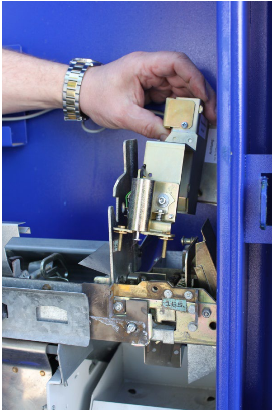
Remove credit device upwards
