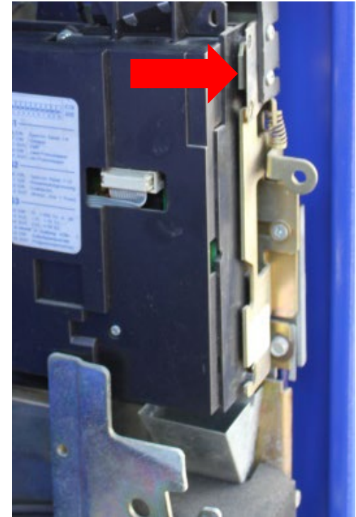
Unlock coin receiver by pulling out the perforated metal plate. Move coin receiver towards the top left.
