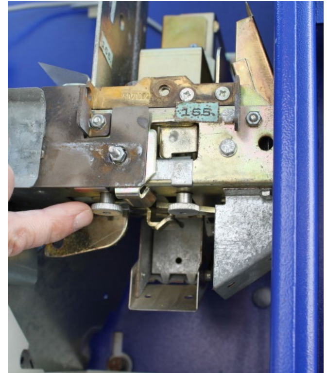
Loosen screw connection
