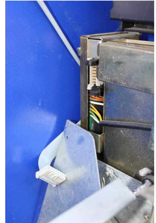
Disconnect the cable (to the coin receiver) at credit device
