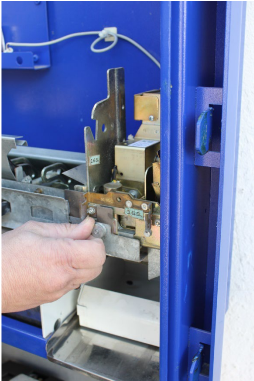
Loosen the screw and remove slice in order to dismantle the coverplate
