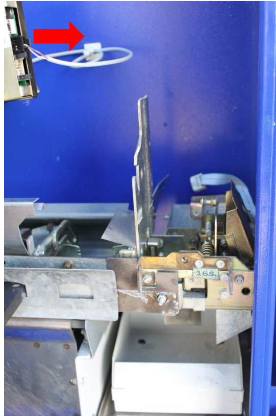
Loosen the plug connection
